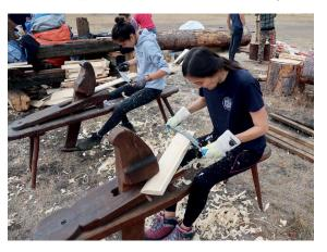
Then you start using a drawknife to finalise the shape of shingle into the ideal proportion, careful to craft a straight surface, without spikes. Master Kai taught us how to feel the surface of a correct shingle and how to replicate it through shaping. The best shingle is one that does not have branch nodes and tissues breaks, which means that the natural structure of the tree is not damaged. Meanwhile machine-made shingles last only for ten years and soon start to rot; correctly handmade
