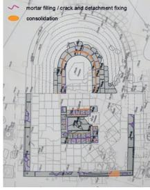
We started with mechanical cleaning of the area. Vegetation and dirt were removed, and we got a clear picture where to focus our future efforts. Due to the mechanical cleaning more cracks were revealed, and these were marked on the technical drawing. The next step was the consolidation of the material structure. Because of the annual changing of climate conditions, the lime mortar that holds the blocks was crumbling because the binder had lost
