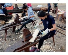
Then you start using a drawknife to finalise the shape of shingle into the ideal proportion, careful to craft a straight surface, without spikes. Master Kai taught us how to feel the surface of a correct shingle and how to replicate it through shaping. The best shingle is one that does not have branch nodes and tissues breaks, which means that the natural structure of the tree is not damaged. Meanwhile machine-made shingles last only for ten years and soon start to rot; correctly handmade
